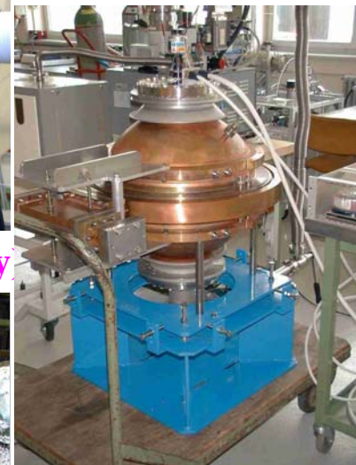
Novel RF power compression with Barrel Open Cavity (BOC)
