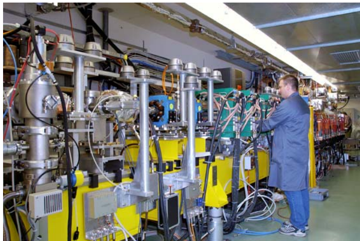
Bunch length adjustment with magnetic chicane
